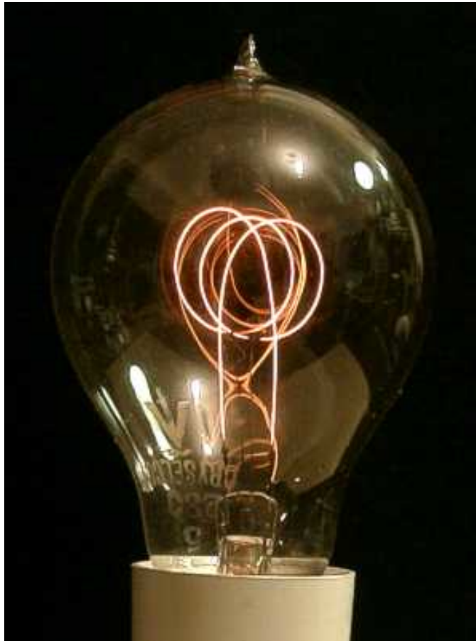
Carbon-filament lamp, Pre-1907.
